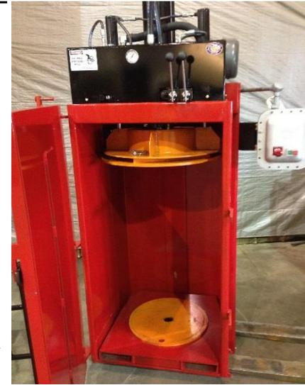
**Universal Head** The squeeze head consists of two easily interchangeable plates. The larger diameter plate is for crushing all sizes of cans and drums. A piercer vents closed drums. The smaller plate is for compacting inside 55-gallon steel or fiber drums. **Compaction Force Control**
